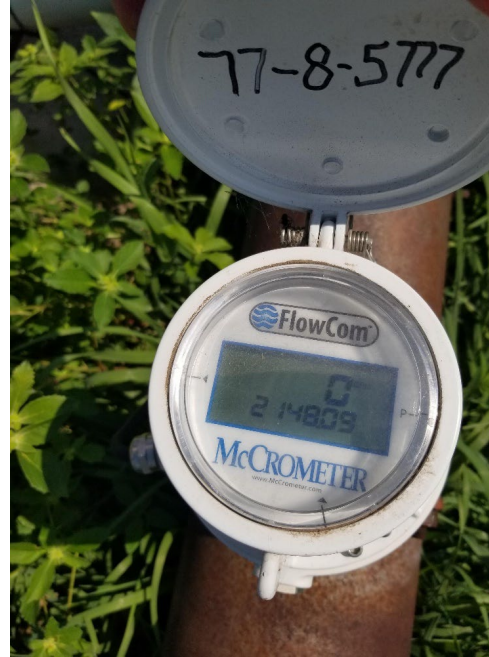
Flow meter with real time telemetry
