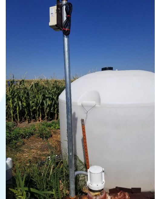
Flow meter with real time telemetry
